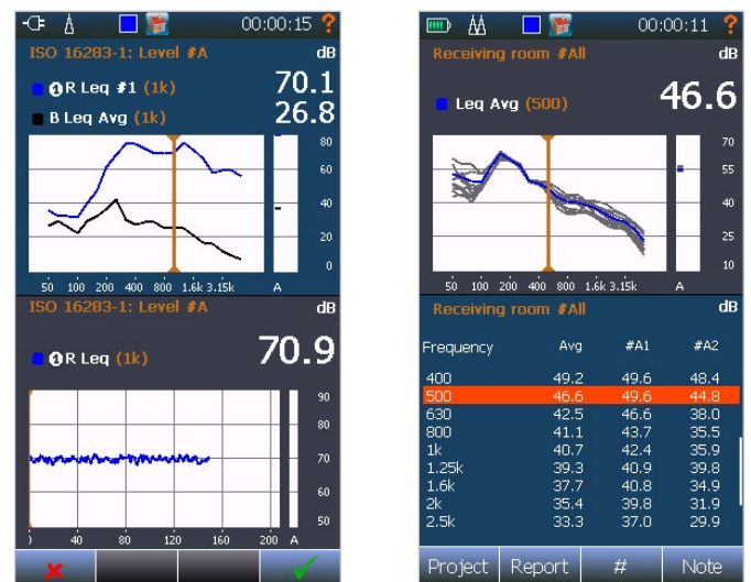
Split screen display (left) with Receiving and Background levels in the upper level versus frequency (L/f) graph. The lower graph is a level versus time presentation of the Receiving room based on the cursor position from the L/f graph. Alternatively, all microphone positions and the average values are displayed together (right).
