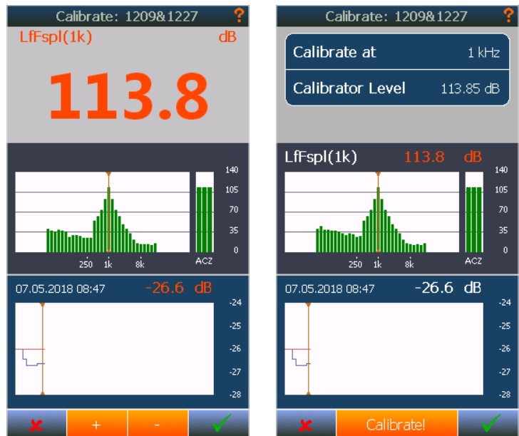
The Calibration menu - Manual and automatic mode
