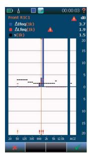
The  $\Delta ext{-view}$  shows the difference between two orthogonal scans
