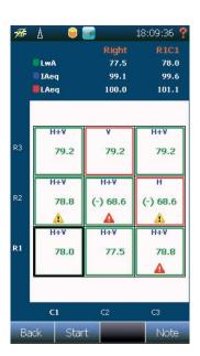
Several segments in a surface. Warnings indicate problems, borders indicate if the segment is completly measured or excluded
