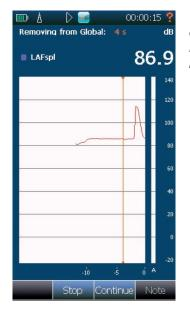
The Pause display allows a chosen number of seconds to be removed from the measurement
